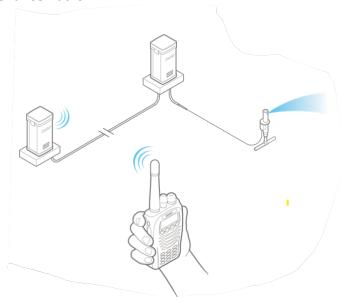
a.) All Hunter Pilot Network systems can use Maintenance Radio remote control with legally licensed UHF radios (Hunter model TRNR, specify frequency). Controllers with PILOT-MOD-UHF radio communications can be addressed directly with StraightTalk™ Technology. No additional steps are required.
